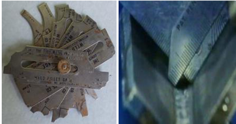
Figure 10. Fillet gauge and its use for measuring leg length
