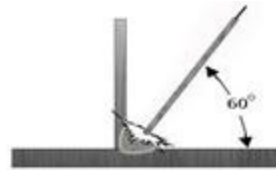
THIN METAL WELDED TO THICK METAL
