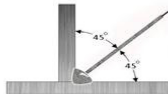
WORK ANGLE FOR SINGLE PASS FILLET WELD
